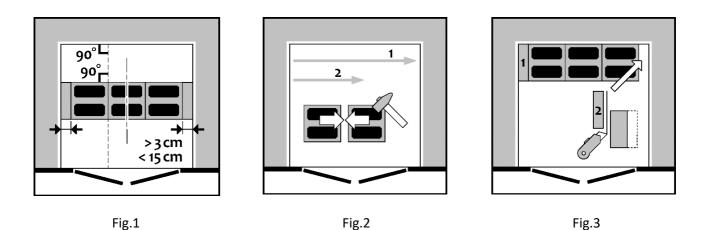
Lay the tiles one row at a time across the width of the mat. Place the second tile in position of the male connector of the first and use a soft headed mallet to lock the tile in place. Repeat with each subsequent tile until the row is complete (see fig. 2)
